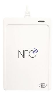
The ACR1552U-MF from ACS is a 13.56 MHz USB-C contactless smartcard reader that supports ISO 14443 type A and B cards, MIFARE, FeliCa, ISO 15693 and ISO 18092-compliant NFC cards and tags. This is the latest evolution of the popular ACR1252, equipped with a SAM slot which provides a high-level of security in contactless and NFC transactions. It boasts faster read/write speeds than previous versions and compatibility with a still wider range of cards.
